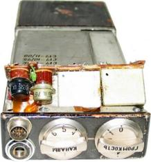
Internal view of top section Angstrem CH, showing controls, aerial socket and remote control socket.
