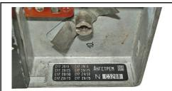
Battery compartment with serial and type number plate showing channel numbers.
