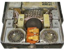
Internal view of top section Angstrem OH showing the two controls and earphone socket.
